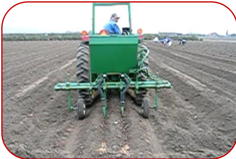
Figure 6.5: A two-row 'Clampco' applicator, banding Multicote™ Agri
