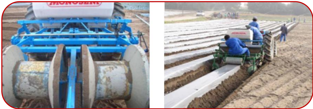
Figure 6.3: A 'Monosem' fertilizer applicator mounted on the ridger. Multicote™ Agri applied simultaneously with bed preparation
