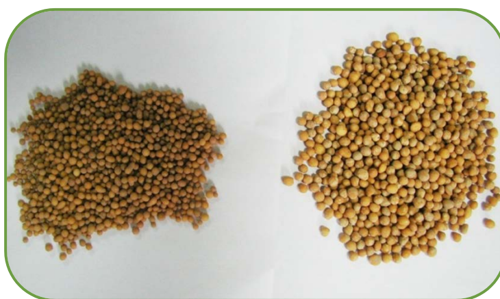
Figure 6.4: Standard CoteN® (left) and non-floating CoteN® (right)
